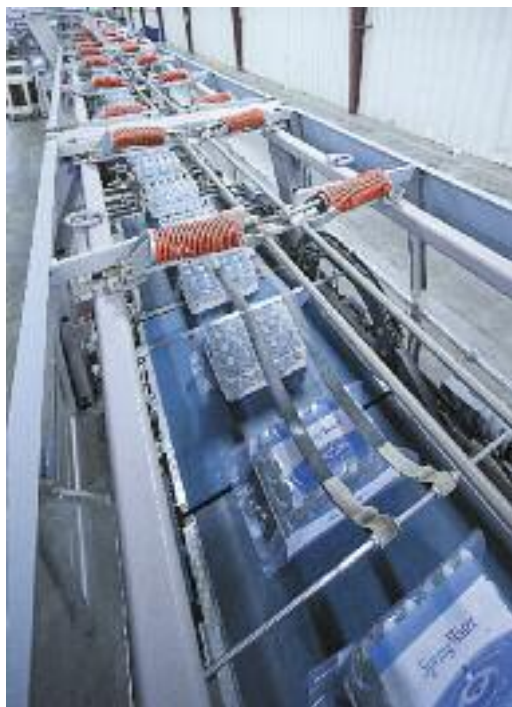
The Innopack Kisters TSP 080 packs 0.5 litre PET bottles in a wide range of formations.
