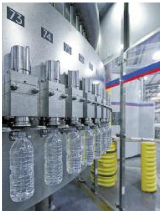
The stretch blow-moulder InnoPET Blomax Series IV monoblocked filling system is geared to Silver Springs' wishes. This is the electronically-controlled normal pressure filling system Innofill NV, on which the non-contact filling via a free-flow filling valve ensures microbiological and hygienic safety.
