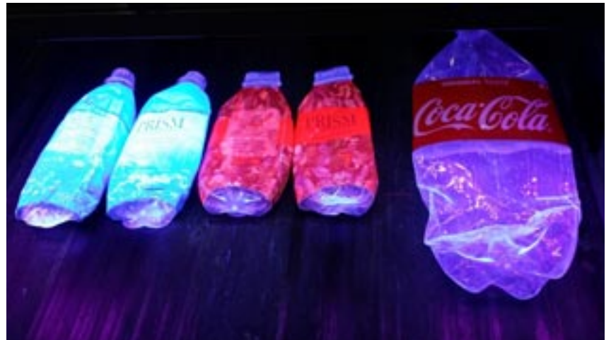
Fluorescent markers – produced from materials recovered from fluorescent lamp recycling and non-rare earth based compounds – are printed on labels or plastic packaging sleeves.
